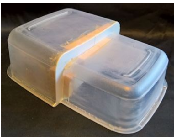
Figures 3.2 – 3.3 The two halves glued to a plasticard plate, outside and inside.
